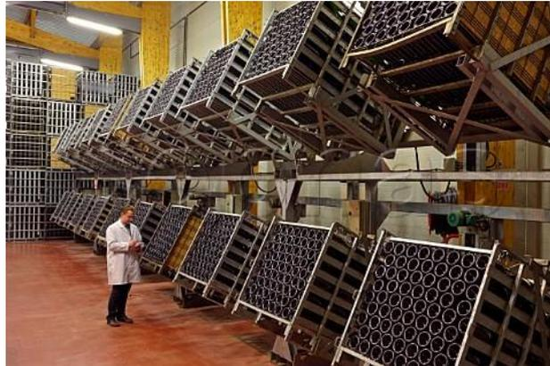
Figure 2. Gyropallets used for automated riddling
